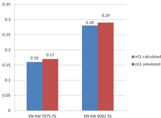
**Fig. 4** Critical nCL values given from physical experiments and numerical simulations
