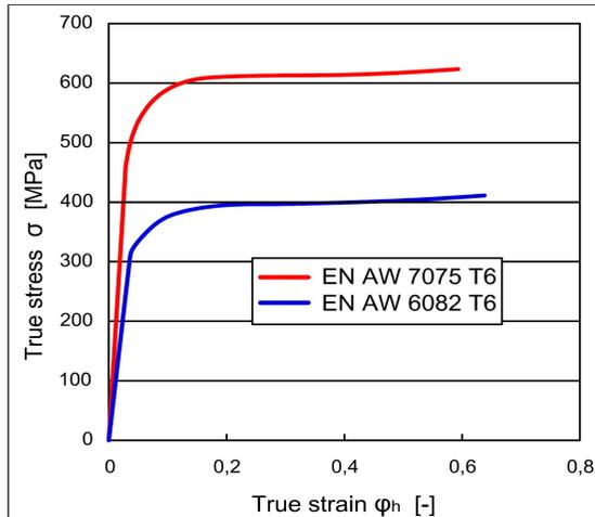
**Fig. 2** Compressive stress - strain curves
