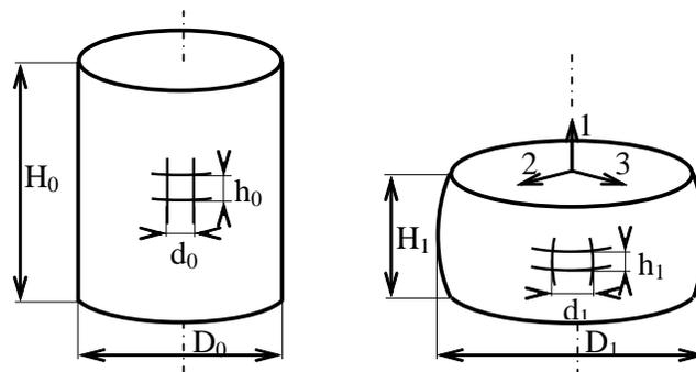
**Fig. 1** Schematic illustration of upset tests showing the grids for strain measurement
