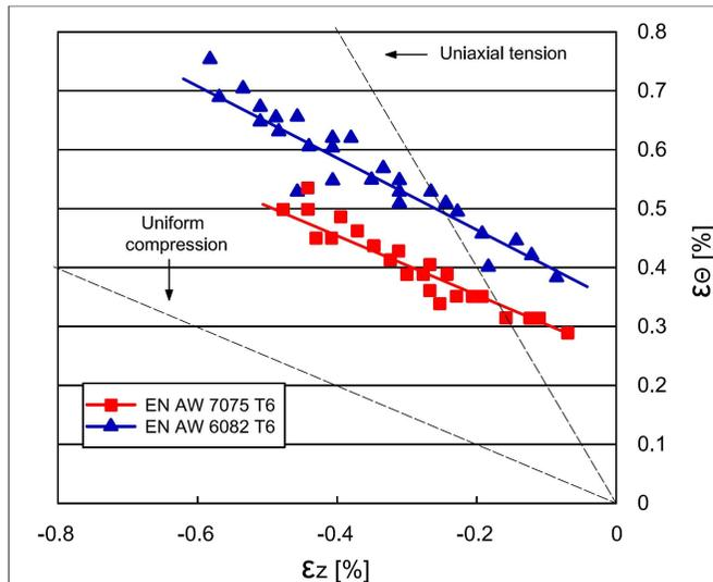
**Fig. 3** Forming limit diagram
