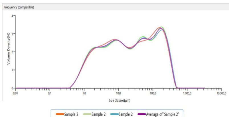
Fig. 4 The particle size distribution for heat treatment regime with number 2 (270 minutes grinded)
