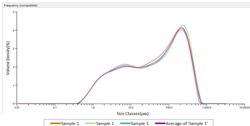
Fig. 2 The particle size distribution for heat treatment regime with number 1 (60 minutes grinded)
