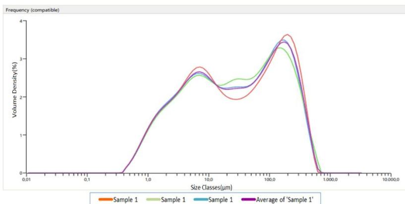
Fig. 3 The particle size distribution for heat treatment regime with number 1 (210 minutes grinded)
