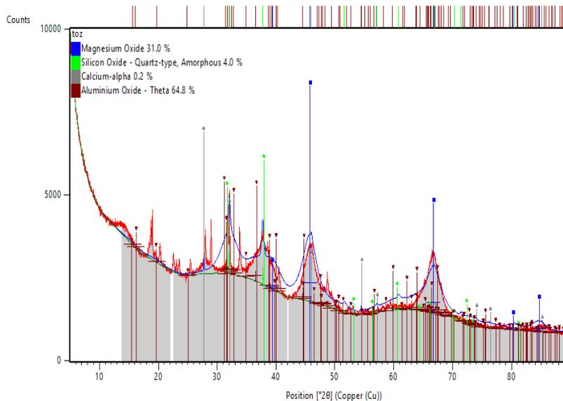
Fig. 1 XRD Analysis of anodized waste sludge
