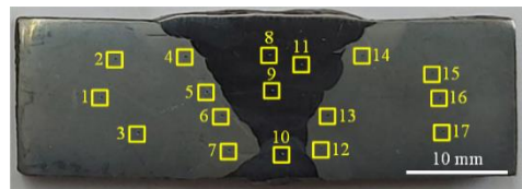
Fig. 3 Presentation of the 14-consecutive passes of TIG welding process and 17 - locations of hardness indentations
