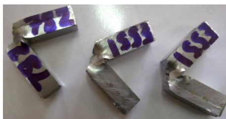
Fig. 7 Impact toughness specimens of the PM after testing at 0 °C
