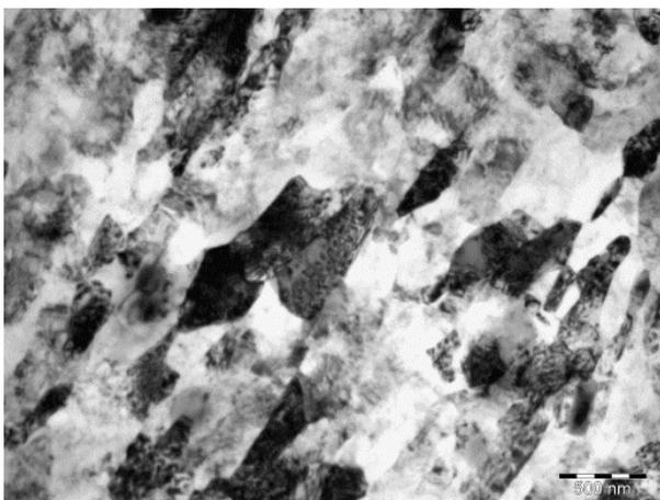
**Fig. 9** Microstructure observed by TEM in post-ECAP artificial aging
