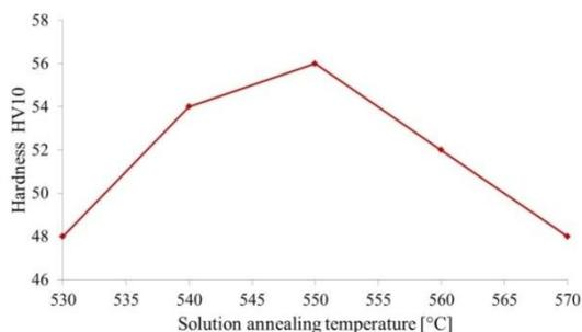
**Fig. 1** Influence of solution annealing temperature on the hardness HV10
