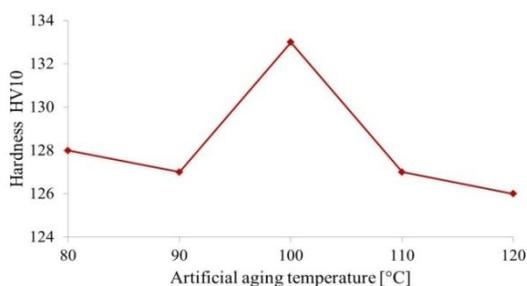
**Fig. 3** Influence of artificial aging temperature on the hardness HV10
