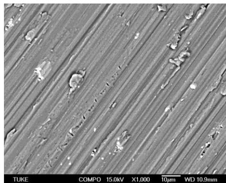
**Fig. 15** Surface after abrasion wear of post-ECAP artificial aging
