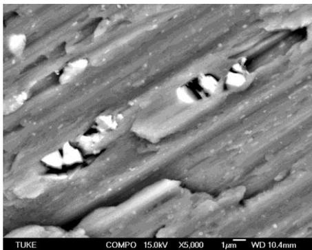
**Fig. 16** Surface detail after abrasion wear of initial state
