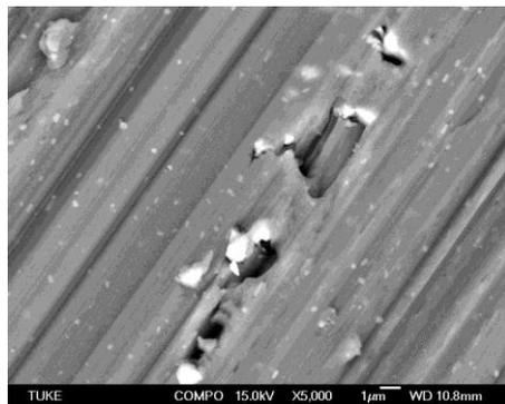
**Fig. 17** Surface detail after abrasion wear of post-ECAP artificial aging
