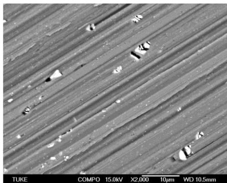
**Fig. 14** Surface after abrasion wear of initial state
