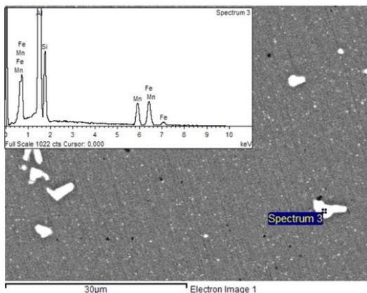
**Fig. 6** EDX analyses of AlSi1MgMn in initial state
