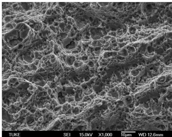
**Fig. 12** Fracture surface of post-ECAP artificial aging
