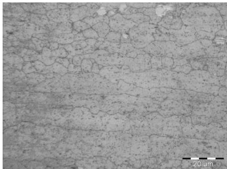
**Fig. 4** Microstructure of AlSi1MgMn in initial state
