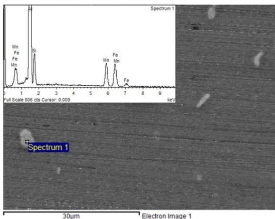
**Fig. 7** EDX analyses of AlSi1MgMn in post-ECAP artificial aging
