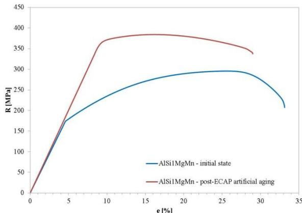
**Fig. 10** Tensile stress-strain curves of initial state and post-ECAP artificial aging
