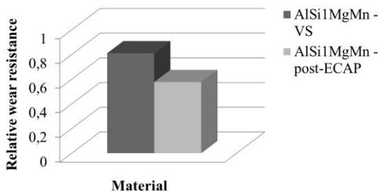
**Fig. 13** Relative abrasive wear resistance of AlSi1MgMn
