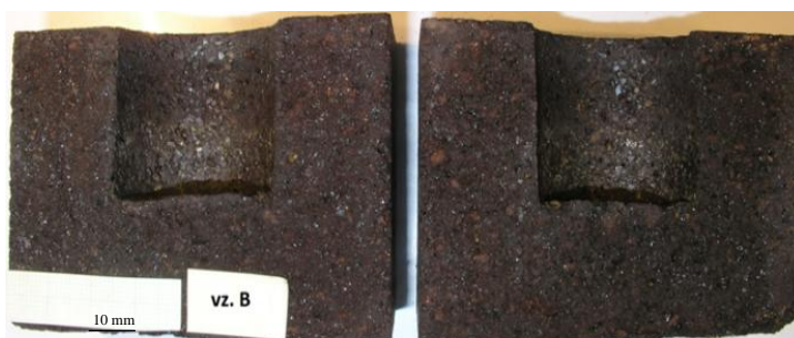
Fig. 2 Macrostructure of magnesia-chromite refractory (B) after the corrosion test with the melt of the system \text{CuO-Na}_2\text{O}\cdot 2\text{SiO}_2
