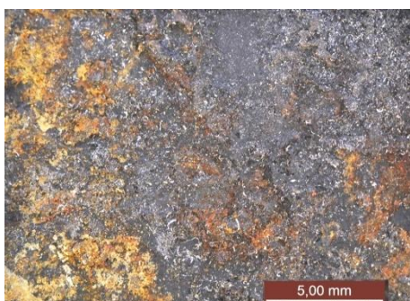
Fig. 4 Steel surface state with protection corrosion layer before exposure in the soil
