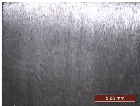
Fig. 2 Steel surface state without corrosion layer before exposure in the soil
