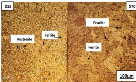
**Fig. 3** Microstructures of the dissimilar weld of duplex stainless steel with X70 steel, joined by solid-state diffusion bonding process at 1150 °C for 5 h.
