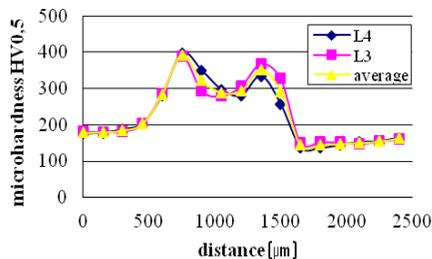
**Fig. 5** Cross weld microhardness profile of S420 and IF laser welded steel sheets
