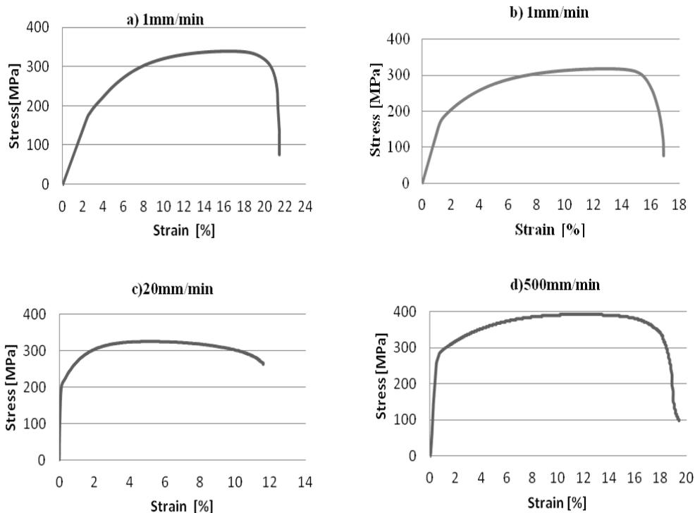
**Fig. 3** Dependence force of IF and S420 steel sheets at time in static condition: a) 1 mm/min, b) 1 mm/min, c) 20 mm/min, d) 500 mm/min
