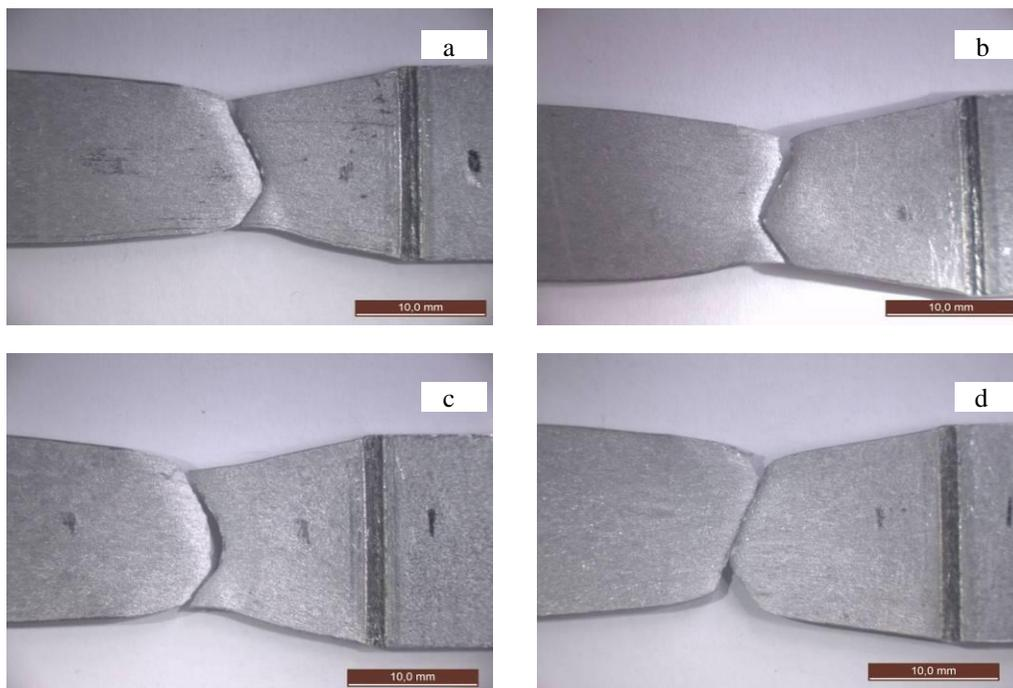
**Fig. 2** Macrostructure laser welded automotive steel in static condition (a, b) mm/min, (b) 500mm/min, (c) 20mm/min
