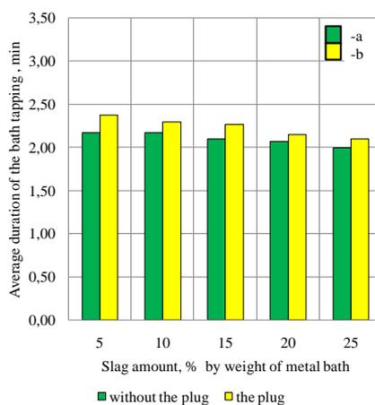
**Fig. 5** Influence of the metal-water tapping option and the amount of slag-oil on the surface of the bath tapping time for (a) tapping without the plug; and (b) with the plug at different amounts of slag-oil on the bath surface.
