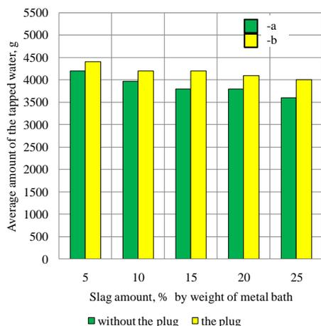
**Fig. 6** The average amount of tapped water-metal according to the experimental options for (a) tapping without the plug; and (b) with the plug at different amounts of slag-oil on the bath surface.
