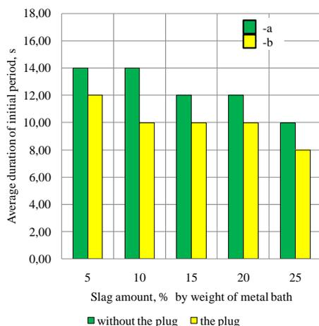
**Fig. 4** Influence of the variant of bath tapping on the duration of the initial period for (a) tapping without the plug; and (b) with the plug for different amounts of slag-oil on the bath surface.
