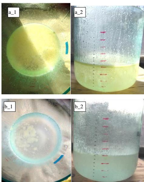
**Fig. 7** Images of the ladle after tapping the bath in the case of a 20% slag layer on the surface of the bath in the converter before tapping, when tapping (a) without using the plug; and (b) using the plug (1b is a top view, 2b is a front view).
