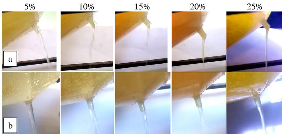
**Fig. 3** Images of the initial period of bath tapping with different amounts of oil-slag on the surface (5-25% of the mass of metal-water) in the case of tapping the bath without the plug (a) and with the plug (b)
