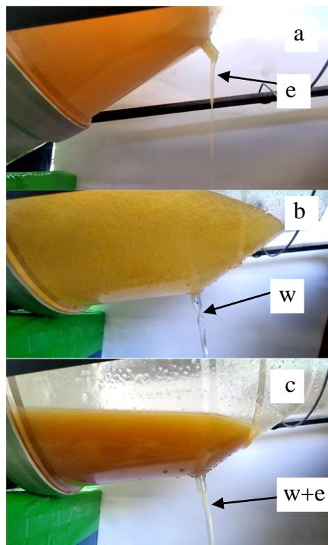
**Fig. 2** Images of bath tapping periods (a) start with emulsion movement; (e), (b) main one with water-metal tapping (w); (c) the final period with the appearance of an emulsion in a jet of water (e+w)
