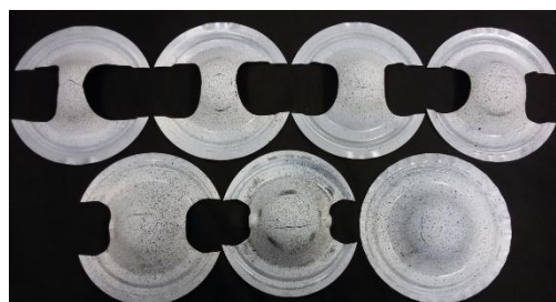
Fig. 4 Dog bone shaped specimens with stochastic pattern after Nakajima test
