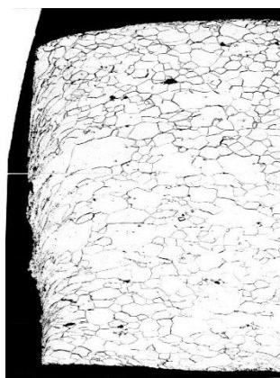
Fig. 7 Microstructure in the cutting area of material C a) cutting gap 0.006mm b) cutting gap 0.012mm enlarged 500x
