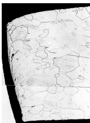
Fig. 6 Microstructure in the cutting area of material A a) cutting gap 0.006mm b) cutting gap 0.012mm enlarged 500x
