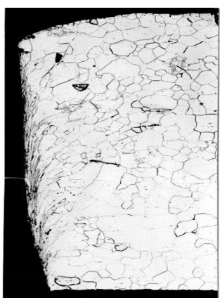
Fig. 6 Microstructure in the cutting area of material A a) cutting gap 0.006mm b) cutting gap 0.012mm enlarged 500x
