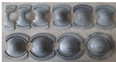
Fig. 13 Samples after the stretch test - determination of residual austenite in the crack area
