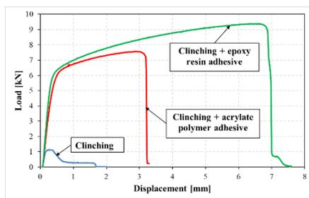
Fig. 6 Load-displacement curves of clinched joint, clinch-bonded joint with acrylate polymer adhesive and clinch-bonded joint with epoxy adhesive
