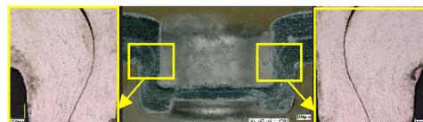
Fig. 7 Cross-section of pure clinching joint with marked area of interlocking
