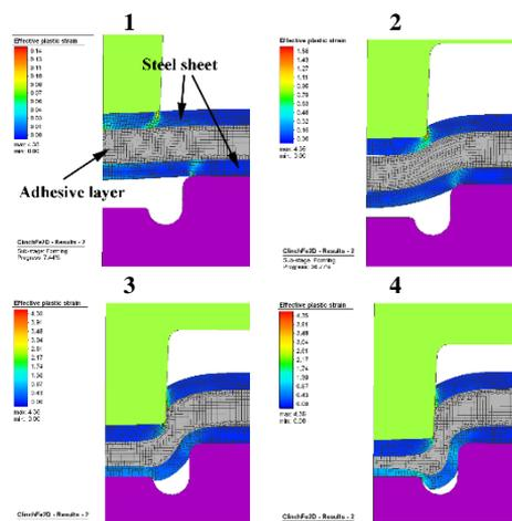
Fig. 5 Clinch-bonding simulation: clinching and acrylate polymer adhesive
