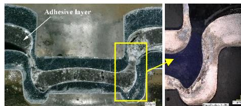
Fig. 8 Cross-section of clinch-bonded joint with epoxy resin adhesive; marked area of interlocking
