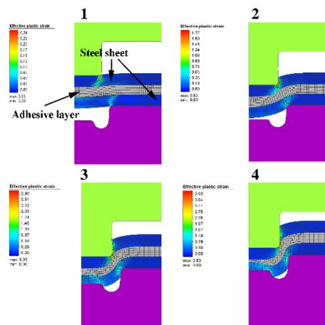
Fig. 4 Clinch-bonding simulation: clinching and epoxy adhesive
