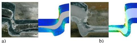
**Fig. 10** Cross-section of clinch-bonded joints: a) with epoxy resin adhesive, b) with acrylate polymer adhesive
