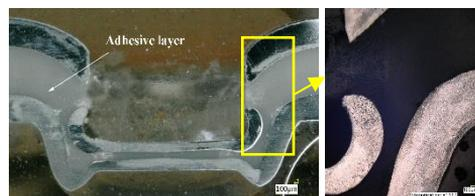
Fig. 9 Cross-section of clinch-bonded joint with acrylate polymer adhesive; marked area with a failure in the interlocking
