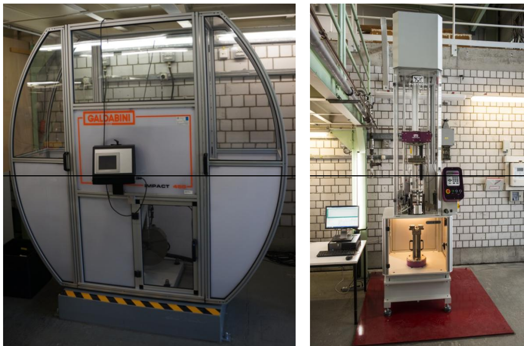
Fig. 3 Charpy Impact Test devices (left: Galdabini 450, right: Instron Ceast 9350)
