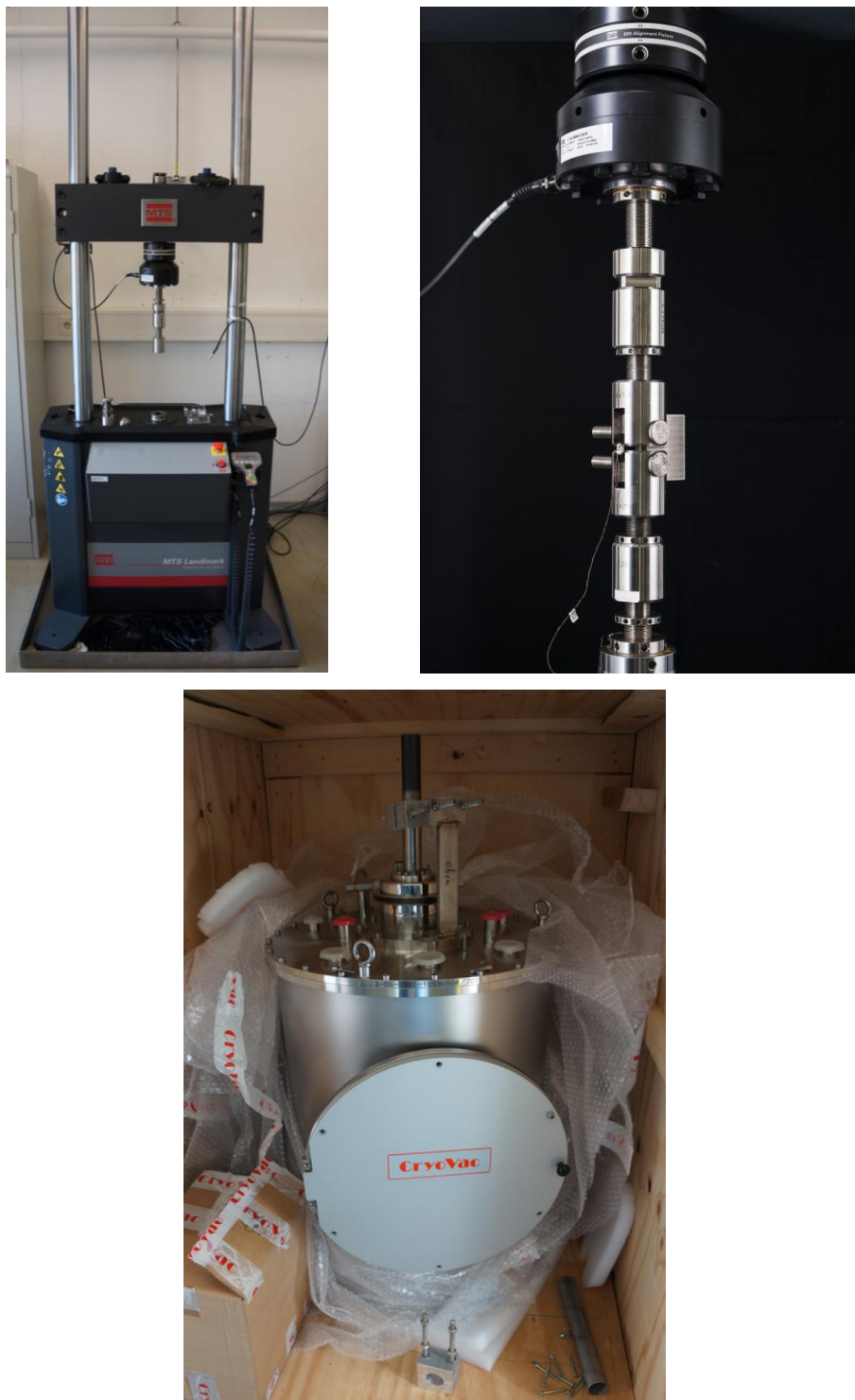
Fig. 2 MTS 100 Landmark with the cryostat (RT → 4K)
