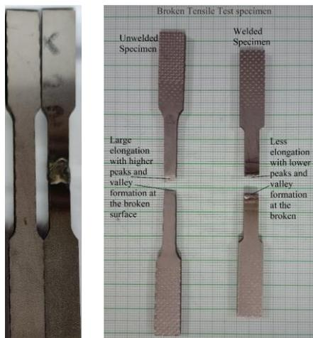
Fig. 2 Tensile test specimens- before and after tension test
