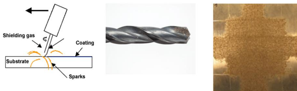
Fig. 1 Principal scheme of ESD process [8] and examples of possible deposition of coating by ESD method at desired surface areas - \text{TiB}_2 deposited on HSS steel drill cutting edge (middle) or on steel plate (right)
