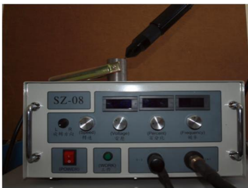
Fig. 2 ESD equipment SZ-08 for electro spark deposition
