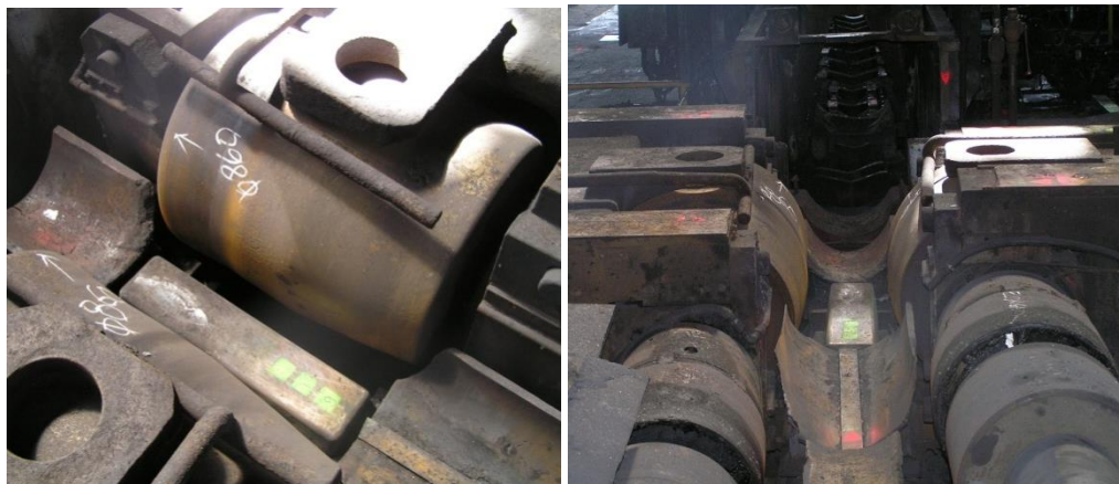
Fig. 2 The photographs of piercing mill in the line for seamless tubes production
