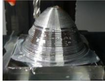
**Fig. 9** Finish operation: Spiral-circle strategy – real machining
