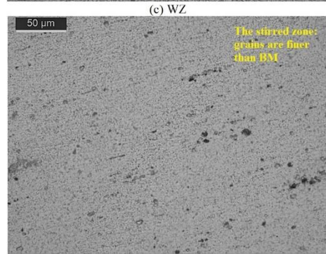
Fig. 10 Microstructural observation in FSW plate
