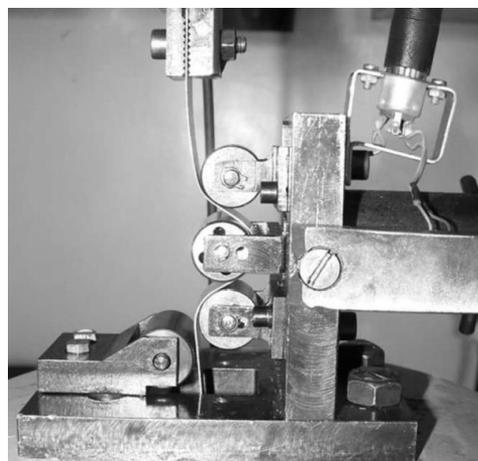
**Fig. 2** Photograph of the friction tester
