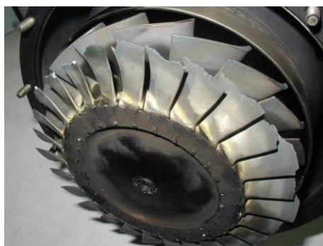
Fig. 1 a, b Appearance of the turbine disc and one destroyed blade with cutting planes (“1, 2”)
