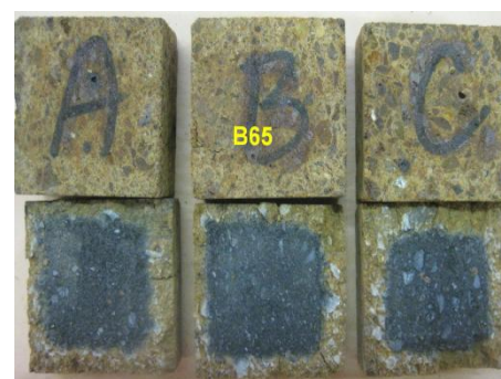
Fig. 4 Oxidation resistance of B65 specimen
