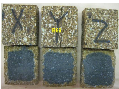
Fig. 3 Oxidation resistance of B66 specimen
