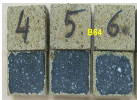
Fig. 1 Oxidation resistance of B64 specimen
