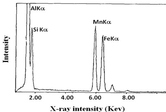
**Fig. 4** X-ray spectrum of a dispersed particles observed in alloy sample ramp heated at 100°C h<sup>-1</sup> to 450°C and water quenched. The main elements are: Al, Si, Mn and Fe
