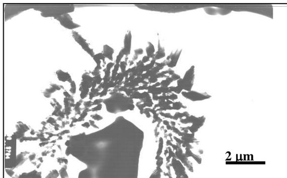
**Fig. 1** Transmission electron micrograph of as-cast alloy showing coarse particles with the plate like and “Chinese script” morphology
