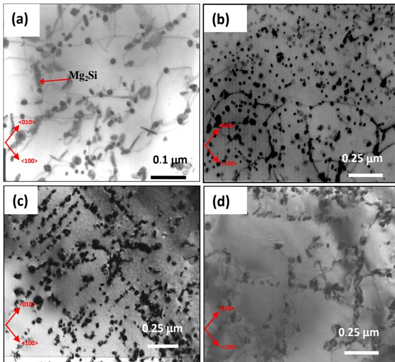
**Fig. 2** Transmission electron micrographs of alloy sample ramp heated at  $100^{\circ}\text{C h}^{-1}$  to  $350^{\circ}\text{C}$  and isothermally aged for : (a) 14 hours, (b) 50 hours , (c) 75 and (d) 120 hours
