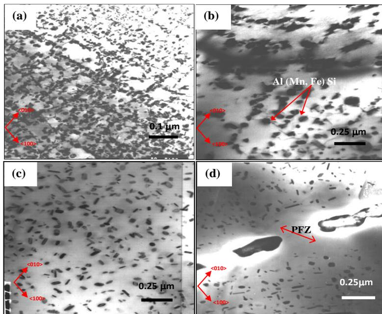
**Fig. 3** Transmission electron micrographs of alloy sample ramp heated at  $100^{\circ}\text{C h}^{-1}$  to  $450^{\circ}\text{C}$  and isothermally aged for (a) 15 hours, (b) 48 hours, (c) 100 hours and (d) 120 hours
