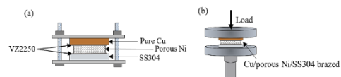
Fig. 1 (a) Samples arrangement (sandwich configuration) in a specific clamp; (b) compression test arrangement in accordance with ISO Standard 13314:2011
