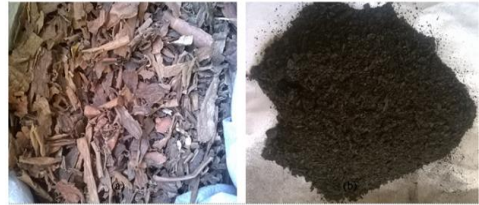
Fig. 1 Cassava-Back-Peel (a) Before Carbonization (b) After Carbonization
