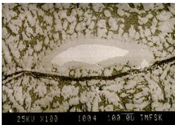
Fig. 6 SEM microphotography of a sample obtained during solid nickel and liquid aluminium interaction ( Fig. 2 , curve 5)
