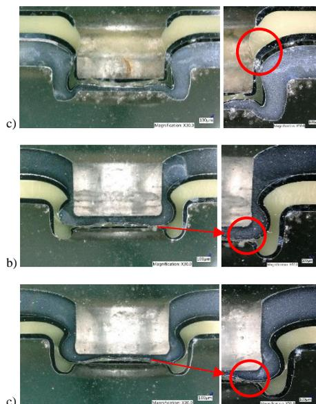
**Fig. 3** Clinched joints: a) Litecor and HCT600X+Z, b) HX420LAD+Z and Litecor, c) HX340LAD+Z and Litecor
