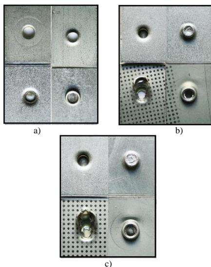
**Fig. 2** The failure modes of the clinched joints: a) Litecor + HCT600X, b) HX420LAD + Litecor and c) HX340LAD + Litecor
