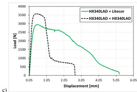
**Fig. 1** The comparison of load–displacement curves: a) Litecor and HCT600X+Z, b) HX420LAD+Z and Litecor, c) HX340LAD+Z and Litecor
