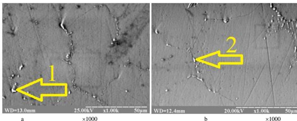
Fig. 5. Morphology of carbides in the structure of the ZhS3DK alloy and points of chemical analysis
