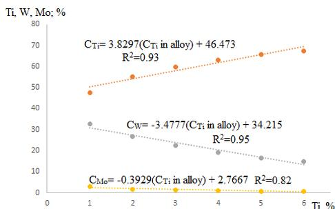
Fig. 2 Dependence of the amount of titanium, tungsten and molybdenum in MC carbides on the titanium content in the alloy
