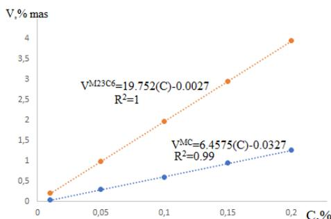
Fig. 1 Dependence of the number of carbides on the carbon content in the alloy composition
