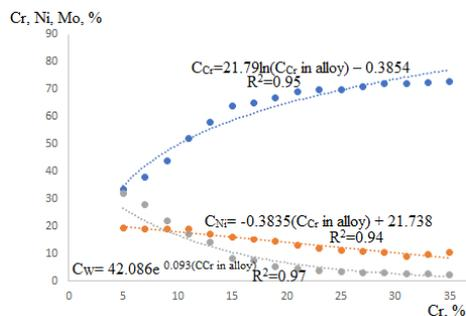
Fig. 4 Dependence of the amount of chromium, nickel and tungsten in  $M_{23}C_6$  carbides on the chromium content in the alloy
