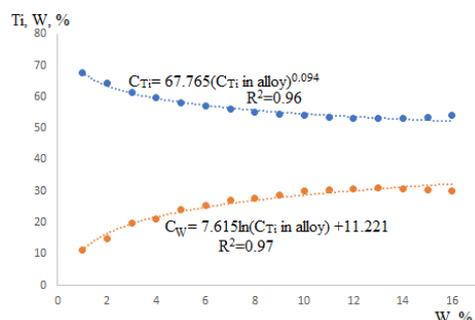
Fig. 3 Dependence of the amount of titanium and tungsten in MC carbides on the tungsten content in the alloy
