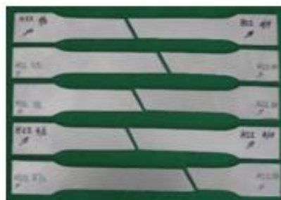
Fig. 2 Test samples of material H22 after uniaxial tensile test, RD = 90°
