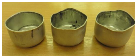
Fig. 10 Cylindrical cups after cupping test
