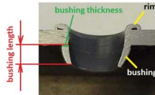
Fig. 3 Cross-section through the axis of a hole produced by thermal drilling
