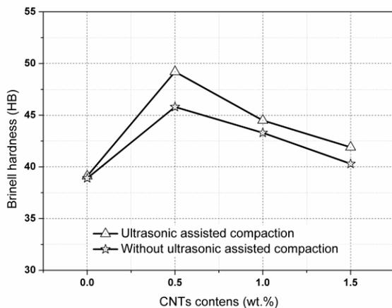
**Fig. 6** Brinell hardness of sintered samples
