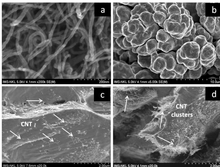
**Fig. 2** FESEM images of a) CNTs, b) Cu powders and c), d) fracture surface of UT.Cu-0.5CNTs after compaction
