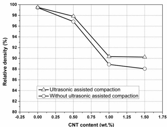
**Fig. 5** Measured density of sintered samples
