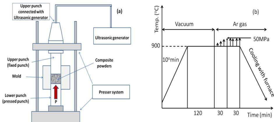
**Fig. 1** a) Scheme of pressing with ultrasonic assisted compaction and b) sinter cycle for sample hot isostatic pressing
