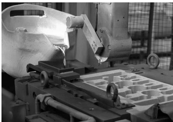
Fig. 1 Production of head cylinder castings – gravity casting
