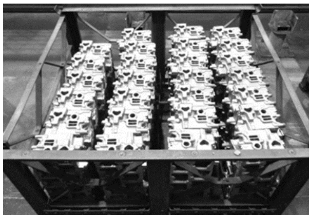
Fig. 9 Positioning of castings in bin
