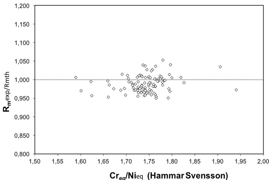
**Fig. 6**  $R_{m\text{exp}}/R_{m\text{th}}$  versus  $Cr_{\text{eq}}/Ni_{\text{eq}}$  calculated according to the classical relationships by Hammar and Svensson [19]
