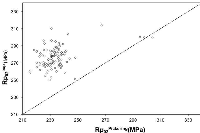
**Fig. 7** Experimental  $R_{p02}$  versus  $R_{p02}$  calculated according to the relationship (2)
