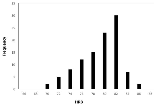
**Fig. 4** HRB of the examined AISI 304 steels
