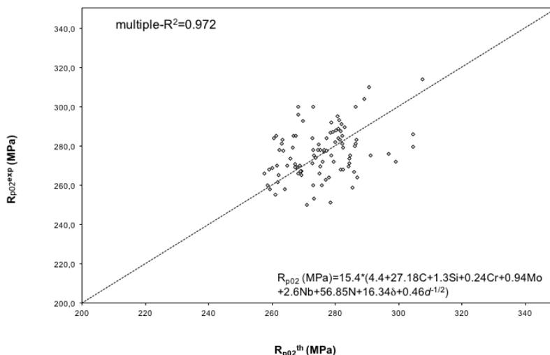
**Fig. 8** Prediction of the 0.2% proof stress according to (3). Multiple- $R^2=0.97$
