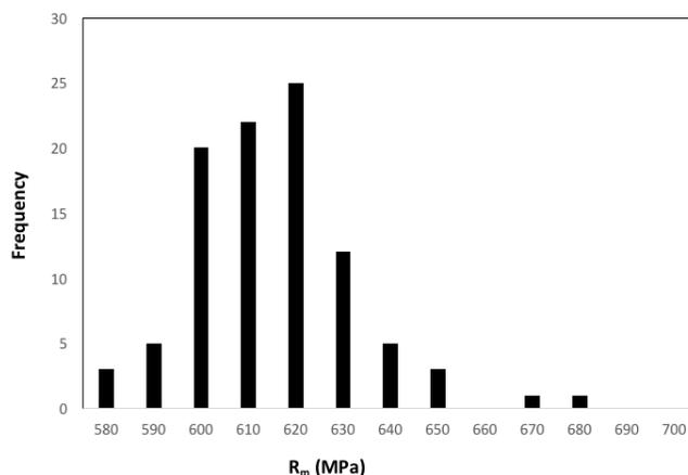
**Fig. 1**  $R_m$  of the examined AISI 304 steels
