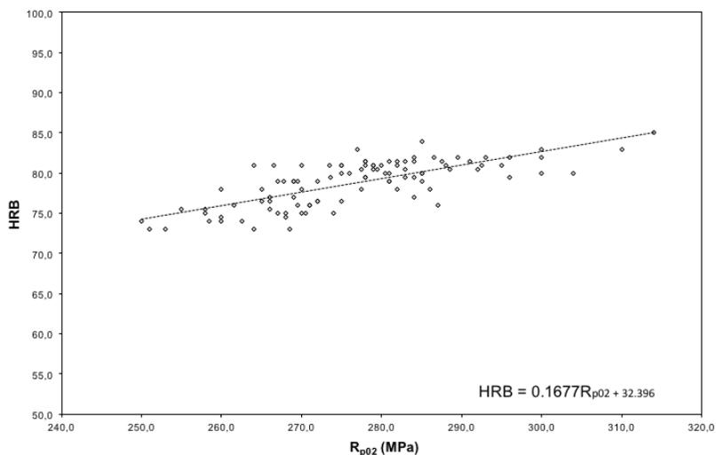
**Fig. 10** Hardness  $HRB$  versus 0.2% proof stress.  $R^2=0.87$
