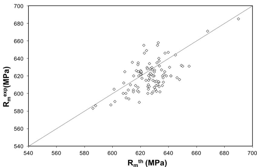
**Fig. 5** Prediction of the tensile stress according to (1). Multiple-R<sup>2</sup>=0.95
