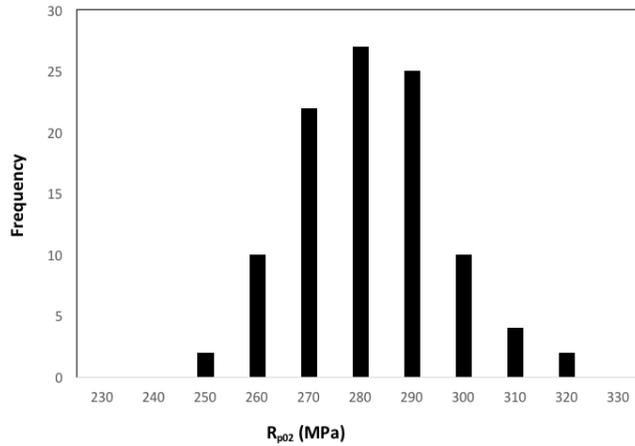
**Fig. 2**  $R_{p02}$  of the examined AISI 304 steels.
