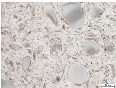
**Fig. 3** Microstructure of ZW3 Mg alloy
