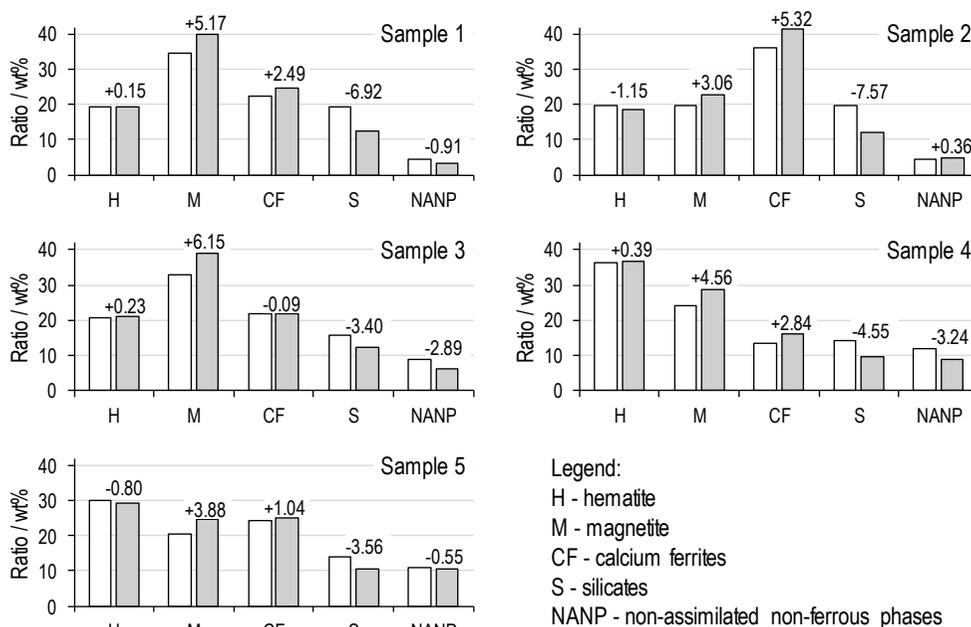
**Fig. 2** Comparison of mineral phases quantification. White and grey columns represent set A and set B, respectively
