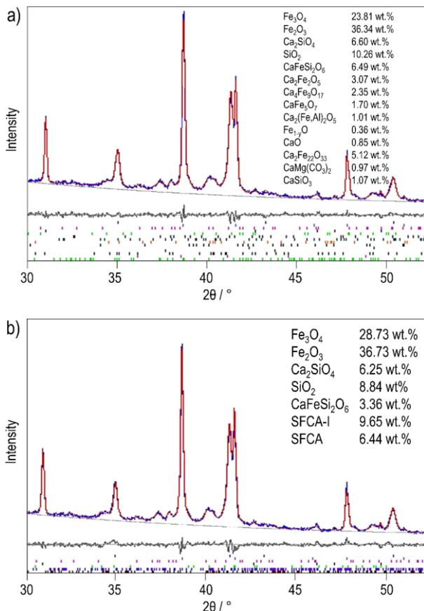
**Fig. 1** Diffractogram of sample 4 within a) set A and b) set B in the range  $30^\circ \leq 2\theta \leq 54^\circ$ . Blue, red, and grey lines represent the measured diffraction pattern, calculated diffraction pattern, and the difference curve, respectively. The list of identified phases corresponds to the order of Bragg reflection markers (online version in color).
