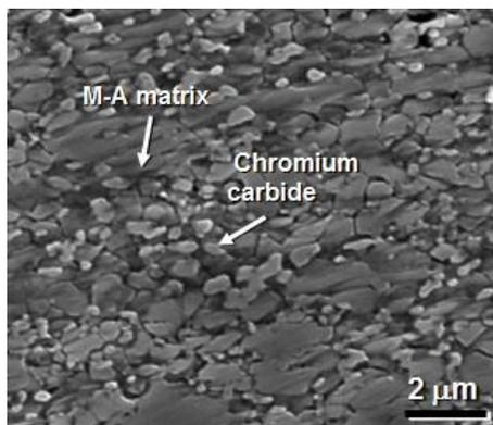
**Fig. 4** Sequence 4 – 1240°C – very fine martensitic matrix with 17% retained austenite and secondary chromium carbides, SEM
