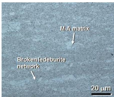
**Fig. 6** Sequence 8 – 1280°C – a larger volume fraction of intact ledeburite network, OM
