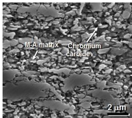
**Fig. 3** Sequence 2 – 1220°C – close-up view of the recrystallized matrix with small islands of coarse unrecrystallized austenitic grains, SEM
