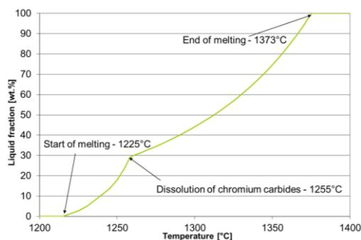
**Fig. 1** Liquid fraction vs. temperature – calculation by JMatPro software
