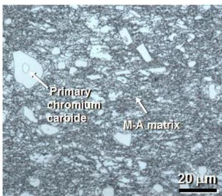
**Fig. 2** Sequence 1 – 1200°C – matrix of fine grains of the M-A constituent with undissolved primary chromium carbides and new precipitates of chromium carbides, OM
