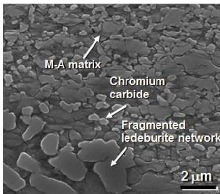
**Fig. 5** Sequence 6 – 1250°C – close-up view of fragmented ledeburite network and martensitic islands, SEM
