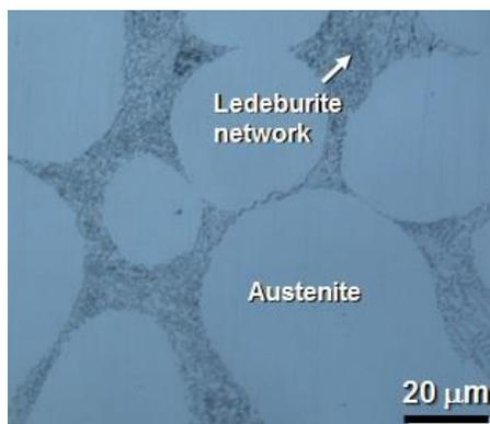
**Fig. 7** Sequence 9 – 1240°C – water quenching – polyhedral austenitic grains with ledeburite network, OM
