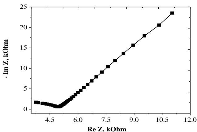
**Fig. 1** Impedance spectrum of compact set from the powder  $\text{ZrO}_2 + 3\text{mol}\% \text{Y}_2\text{O}_3$ ,  $400^\circ\text{C}$ , 2h, obtained from the chloride raw material
