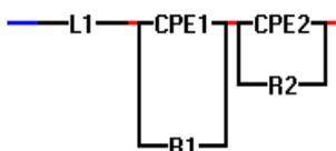
**Fig. 2** Equivalent electrical circuit of the investigated object
