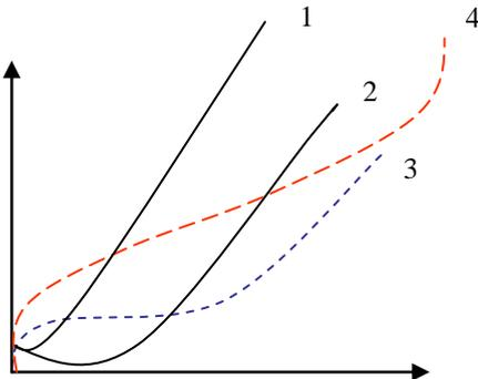
**Fig. 4** Schematic diagram, that reflecting the trend to transformation of impedance of samples during PMF processing: 1 - the initial state; 2 after 45 minutes processing; 3 - after 55 minutes processing; 4 - after 95 minutes of treatment
