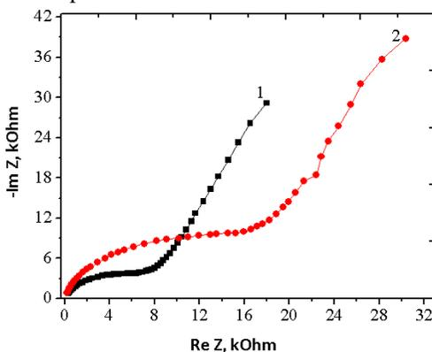
**Fig. 5** Typical spectra of the sample: 1 - before processing by a pulsed magnetic field; 2 - after processing by a pulsed magnetic field in the mode: 10 Hz, 1 hour
