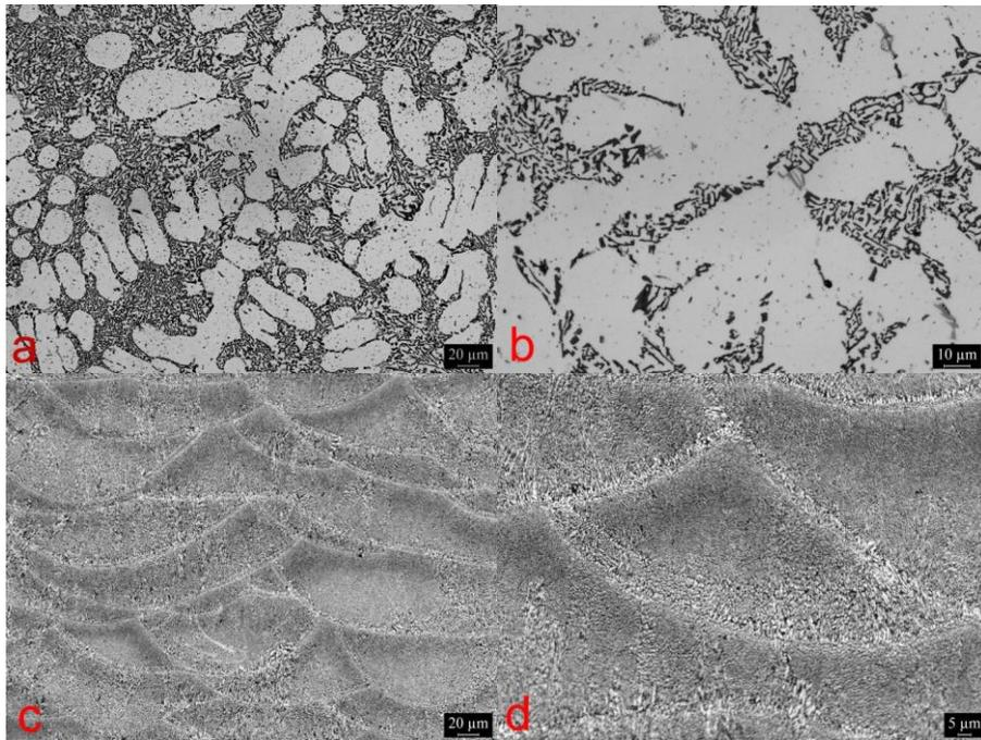
**Fig. 2** Comparison among AlSi10Mg macrostructures obtained through: casting (a-b) and L-PBF process (c-d); the red arrow indicates the building direction, or *z-axis*
