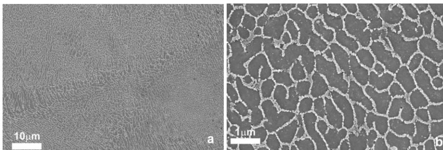
**Fig. 3** FESEM images of AlSi10Mg microstructure by L-PBF process: (a) melt pool borders are visible; (b) a magnification of the melt pool center
