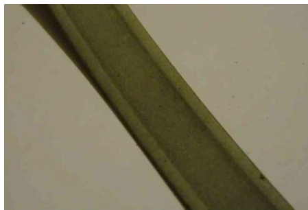
Fig. 7 View of the specimen surface ( w = 20 mm) tested under conditions of dry friction, R_a of rolls equals of 0.63 \mu\text{m} and middle roll displacement h = 18 mm
