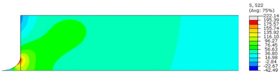
Fig. 11 Tearing S22 stress distribution in the adhesive layer of joint ( F = 5282 \text{ N} , elastic-plastic model of adherend)
