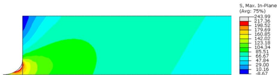
Fig. 10 Maximum principal stress distribution in the adhesive layer ( F = 5282 \text{ N} , elastic-plastic model of adherend)
