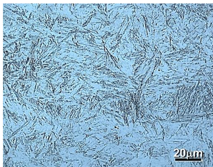
Fig. 6 Martensite with certain fractions of bainite and retained austenite, optical micrograph, interior of the forging
