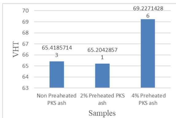
**Fig. 3** Vicker hardness values of the AMCs
