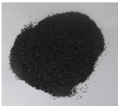
**Fig. 1** PKS ash particles
