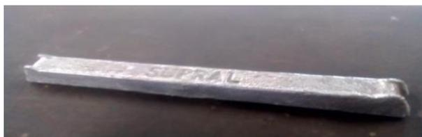
**Fig. 2** Ingot of A16061
