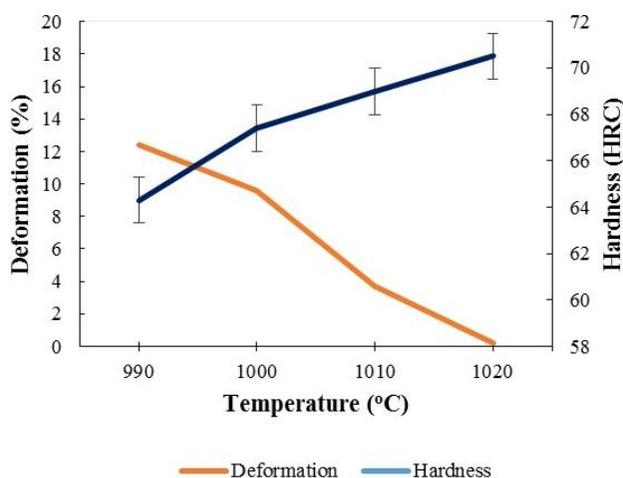
**Fig. 4** The effect of sintering temperature on the mechanical properties of FeMn13-TiC composites with different sintering temperatures
