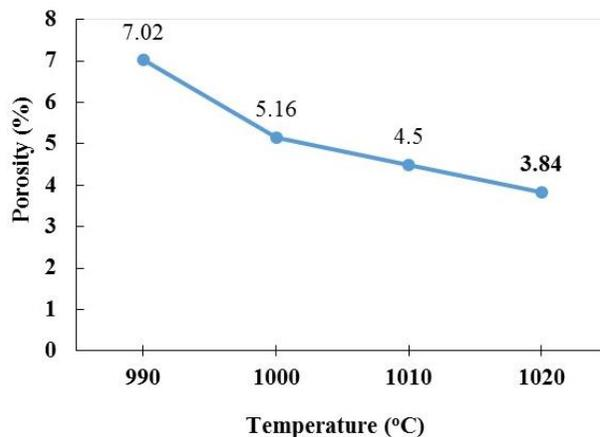
**Fig. 2** The effect of the sintering temperature on the densification of FeMn13 - TiC composites
