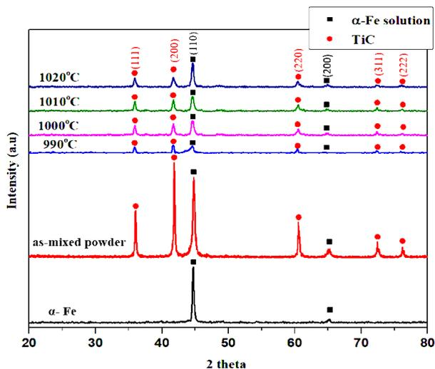
**Fig. 1** XRD patterns of the as-mixed powder and sintered samples
