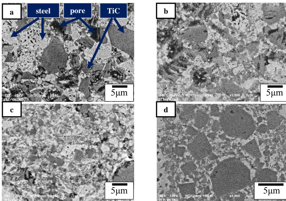
**Fig. 3** Microstructure images of polished samples sintering at different sintering temperatures a. 990°C, b. 1000°C, c. 1010°C, d. 1020°C
