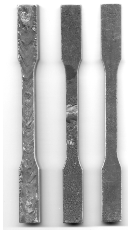
Fig. 2 Tensile specimens - with longitudinal weld (left), with transverse weld (middle) and base material (right)
