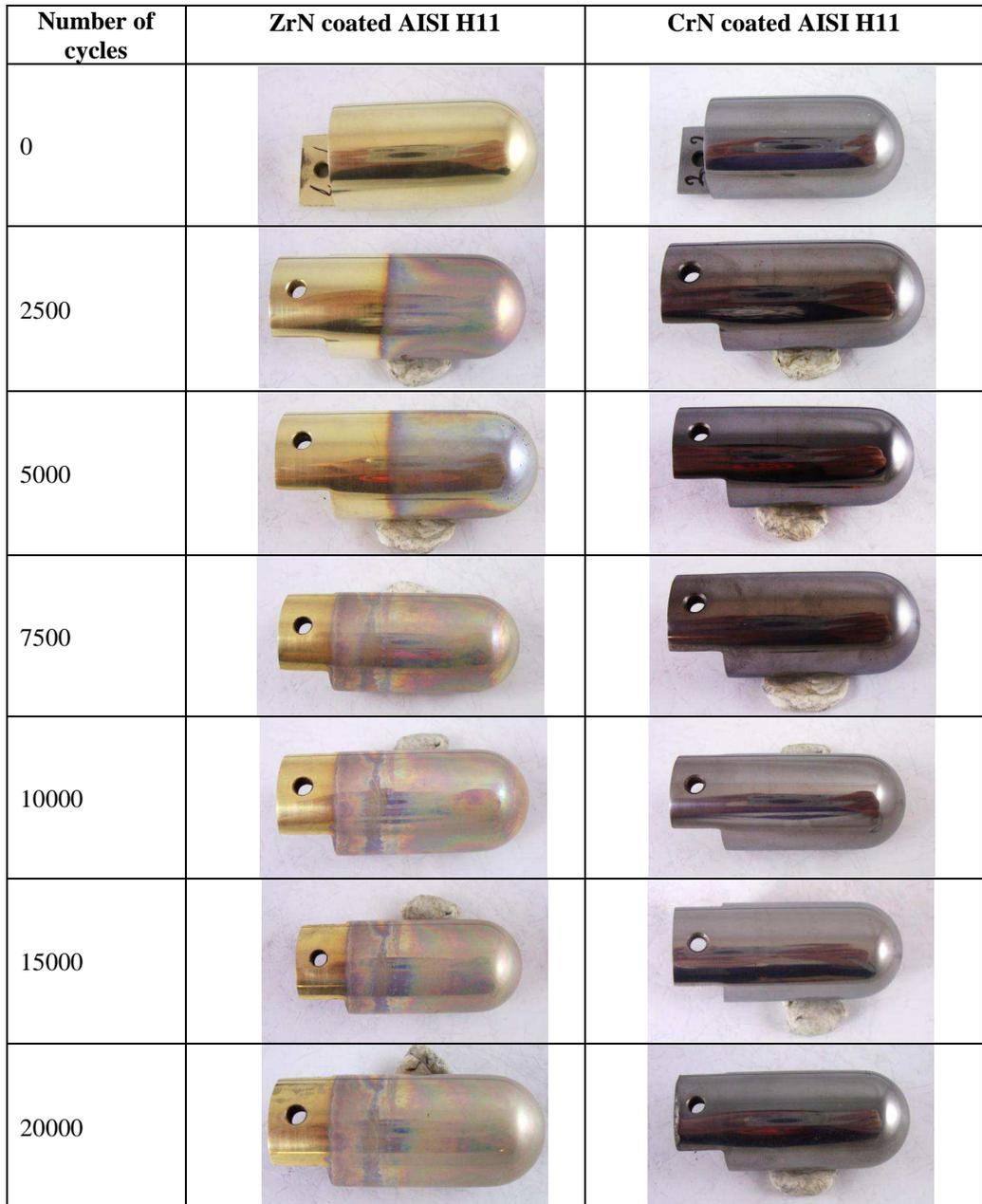
**Fig. 4** Macroviews of the inspection on the CrN and ZrN coated AISI H11 samples at different steps of the cyclic immersion test.
