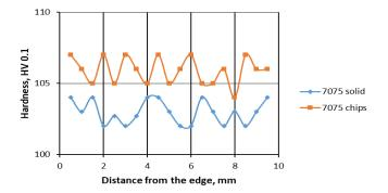
Fig. 6 Hardness distribution in the extrudate made of chips and solid materials by KoBo method
