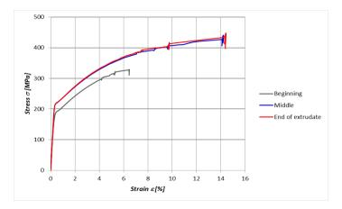
Fig. 4 Tensile curves of  $\varphi 10~\text{mm}$  rods after 7075 chips consolidation by KoBo method
