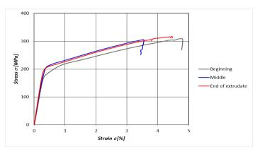
Fig. 5 Tensile curves of  $\phi 10$  mm rods obtained from bulk 7075 materials by KoBo method
