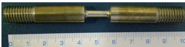
Fig. 1 Sample for SSRT test of stress corrosion cracking
