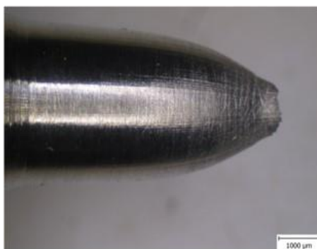
Fig. 9 Example of a sample after SSRT test with typical ‘neck’ of mechanical fracture
