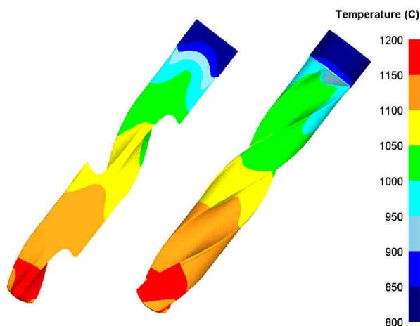
**Fig. 8** Drill temperature distribution in final process stage
