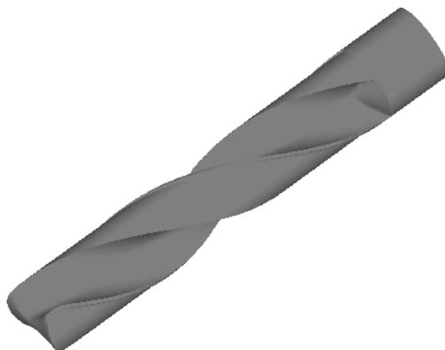
**Fig. 5** Drill forging obtained in FEM calculations
