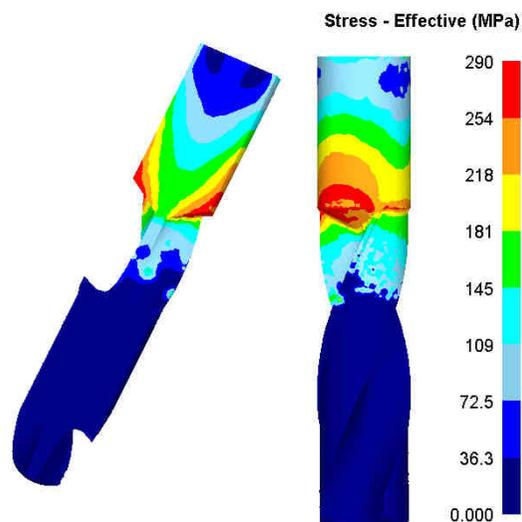
**Fig. 9** Numerically determined distribution of stresses
