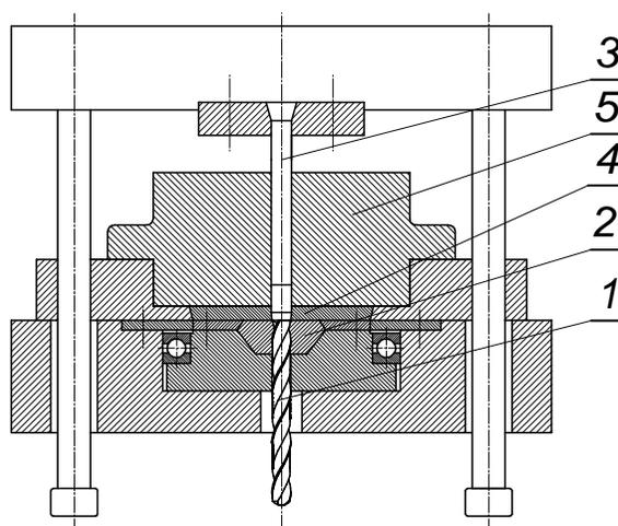
**Fig. 3** Device for twist drill extrusion (described in paper) [12]
