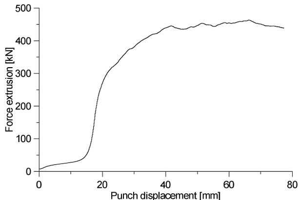
**Fig. 7** Force in twist drill extrusion process
