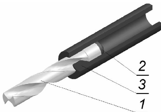
**Fig. 2** Scheme of twist drill extrusion process (described in the paper)
