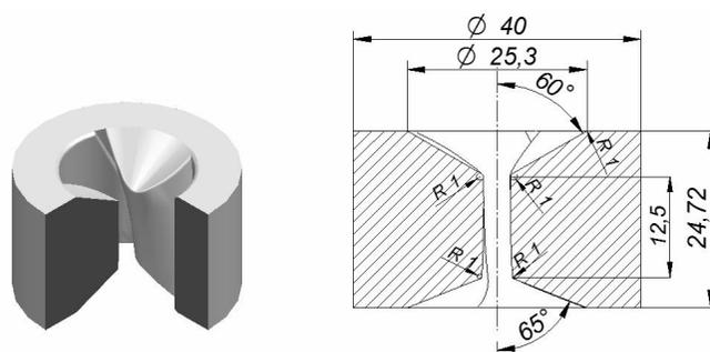
**Fig. 4** Scheme of die used in twist drill extrusion simulation
