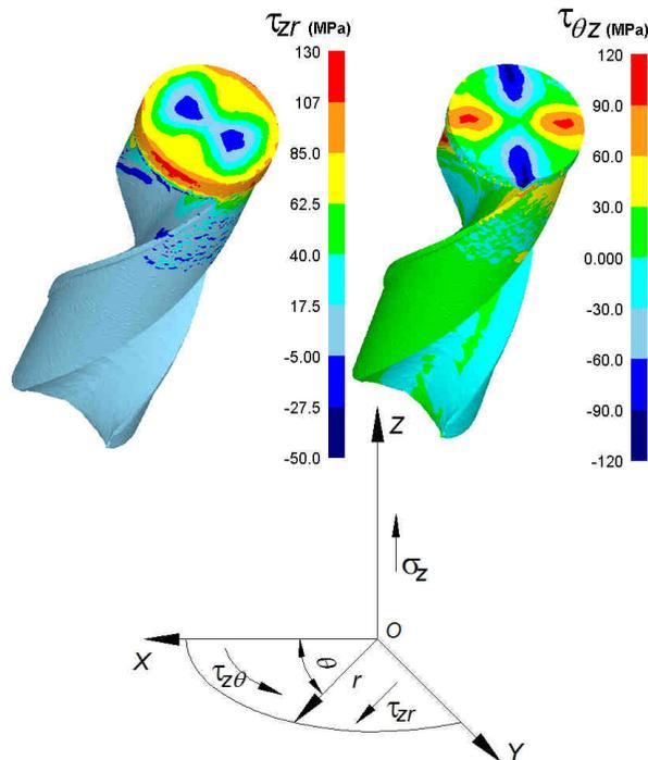
**Fig. 10** Numerically determined shear stresses
