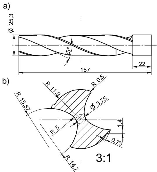
**Fig. 1** Scheme of analyzed drill: a) general view, b) cross-sectional view
