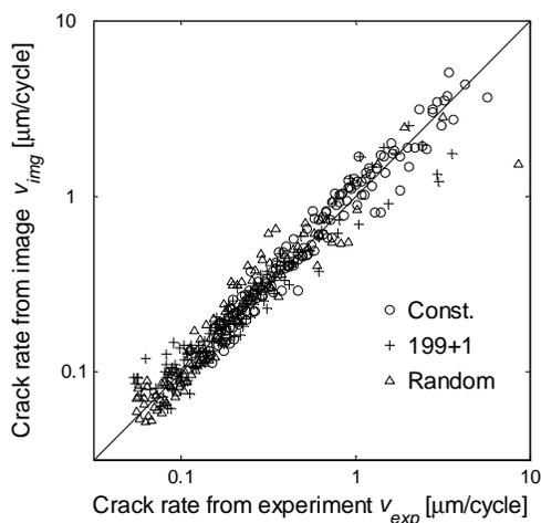
**Fig. 4** Comparison of input (known) and output (estimated from images) crack growth rates. Markers represent single images of the fracture surface.
