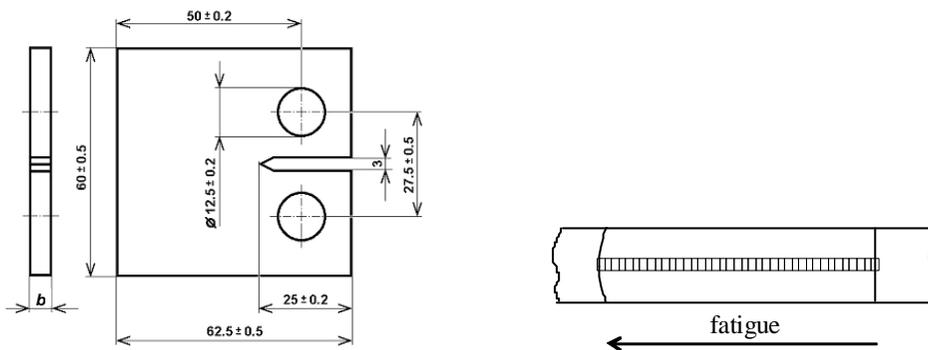
**Fig. 2** Specimen for fatigue tests. **Fig. 3** Layout of SEM images along the middle axis of the fracture surface.
