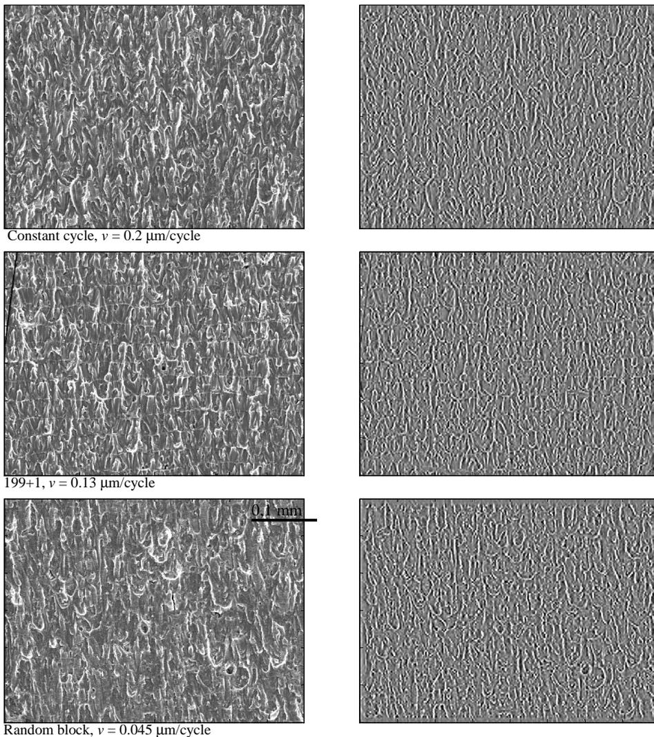
**Fig. 7** a) Normalized SEM images of the crack surfaces. Reference crack growth rate  $v_{ref} = 0.2 \mu\text{m}/\text{cycle}$ . b) Corresponding reference textures.
