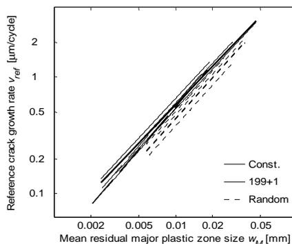
**Fig. 6** The dependence between  $w_M^{1/}$  and the reference crack growth rate  $v_{ref}$ .<sup>2/</sup>
