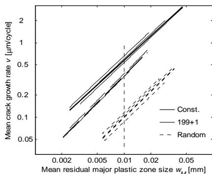
**Fig. 5** The dependence between  $w_M^{1/}$  and the mean conventional crack growth rate  $v$ .<sup>2/</sup>
