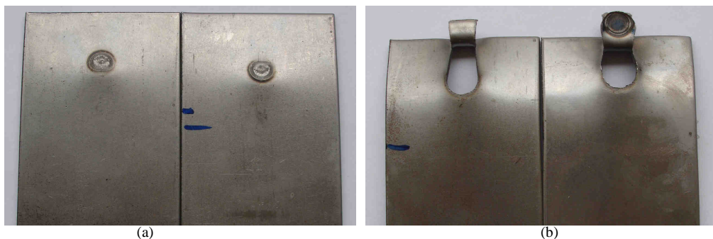
Fig. 2 Observed failure modes during tensile-shear test a) interfacial failure mode b) pullout failure mode
